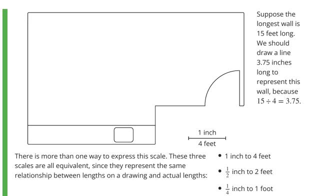
Any of these scales can be used to find actual lengths and scaled lengths (lengths on a drawing). For instance, we can tell that, at this scale, an 8-foot long wall should be 2 inches long on the drawing because  $\frac{1}{4} \cdot 8 = 2$ .
