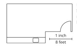
Notice this drawing is smaller than the previous one. Since one inch on this drawing represents twice as much actual distance, each side length only needs to be half as long as it was in the first scale drawing.
