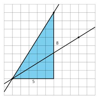
Construct triangles perpendicular to the axes whose hypotenuses lie on their line to find the slopes. The slopes of the lines are then the quotient of the length of the vertical edge by the length of the horizontal edge.
