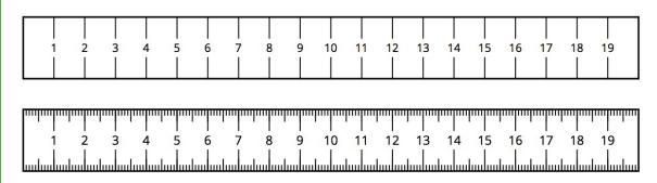
The second ruler is marked in millimeters, so it is easier to get a measurement to the nearest tenth of a centimeter with this ruler than with the first. For example, a line that is actually 6.2 cm long might be measured to be 6 cm long by the first ruler, because we measure to the nearest centimeter.
