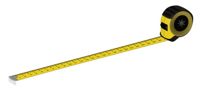
Display the image of the metal measuring tape for all to see. Ask if any students have used a tool like this before, and for what purpose. Tell them that many measuring tapes like this are made out of metal, and that some metals expand or contract slightly at warmer or colder temperatures.
