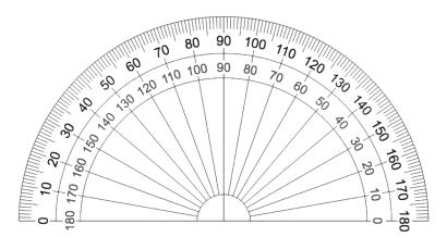
A protractor has two sets of numbers and that either set of numbers could be used, but it is helpful to use the set that counts up from 0 rather than count down from 180. We used a protractor to measure and draw different angles.
